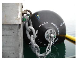
Ocean Guard™ Netless foam filled marine fenders efficiently absorb significant amounts of energy with a low corresponding reaction force, lower than pneumatic or rubber buckling fenders. These Ocean Guard™ Netless foam filled fenders is designed to absorb 225 ft-kips (31 ton-m) of energy when 60 percent compressed with a corresponding load of 167 kips (75 tons).
