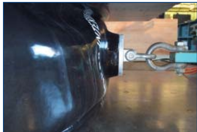
FENDER TESTING AT 60% COMPRESSION In accordance to US Navy specifications
