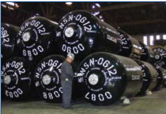
Skin thickness testing on each fender
